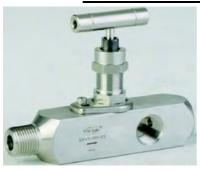
Uni-Lok Gauge Root Valves offer a safe and economical method of installing pressure switches, gauge and differential transmitters. By offering multiple outlets, these valves can accommodate a variety of gauge positions and handle operations. They are suitable for block and bleed where a purge valve, sampling line, or test pressure source is required.
