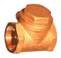
The SWING CHECK VALVE is a low pressure valve mainly for use with water. It should only be used in the horizontal position as it relies on back flow pressure to remain shut.
